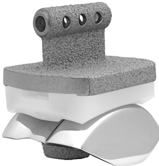
Fig. 1. The Salto Talaris total ankle replacement is a fixed-bearing prosthesis with anatomic design features. The talar component has varying radii of curvature that simulate the mechanical frustum of the ankle with motion. The plasma titanium spray on the surface promotes ingrowth of bone and stable biologic fixation. The keel increases osseous contact.
